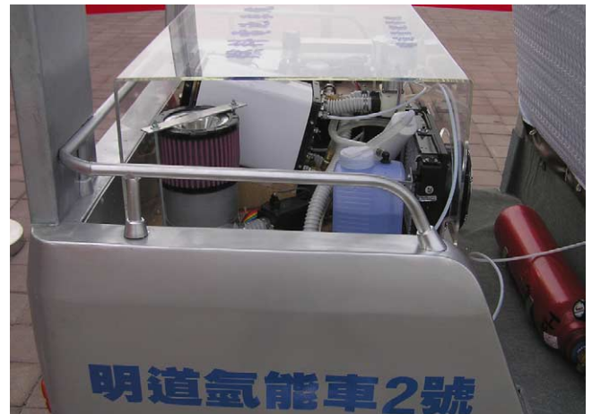
Fig. 6. Installation of fuel cell system on the rear seat of the electric vehicle.
