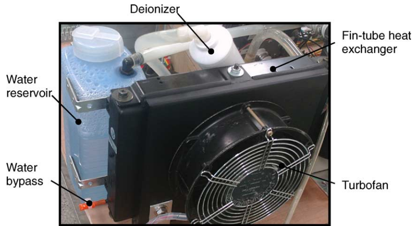
Fig. 4. Cooling subsystem of the fuel cell system (water pump is behind the heat exchanger).
